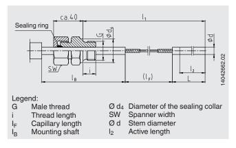
For stem diameter 6 mm no bend protection spring will be fitted at the probe.
